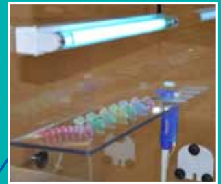
UV light and UV shelf for enhanced irradiation of supplies
