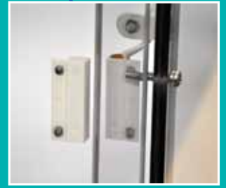
Sash safety switch automatically turns off UV light and activates the blower when sash is raised
